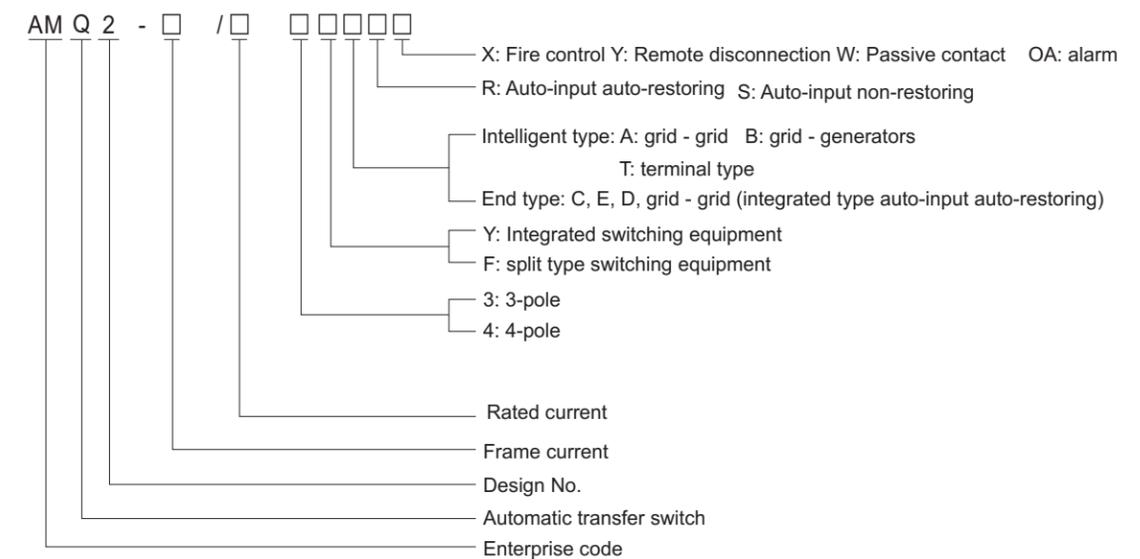
Note: types C, E, D and W provide integrated auto-input auto-restoring only, types C and E have no fire protection, remote disconnection or passive contact.
