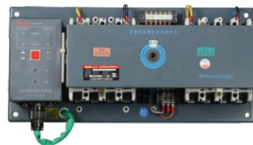
started up automatically and the system will switch to generator set for power supply once the generating voltage reaches normal range (above 80% rated voltage). When the grid voltage returns to normal (above 80% rated voltage), the system will switch back to normal power for power supply again after time delay.
